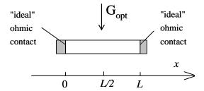
This bar silicon has ideal Ohmic contacts on both sides. Find the excess electron density throughout the material using the simple recombination model and assuming that  $\mu_n = \mu_p = 1000 \text{ cm}^2/\text{V-s}$ .
